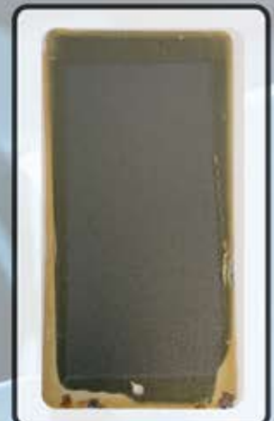
TRS-BEVO3 10 CYCLES - CYCLIC CORROSION TEST
